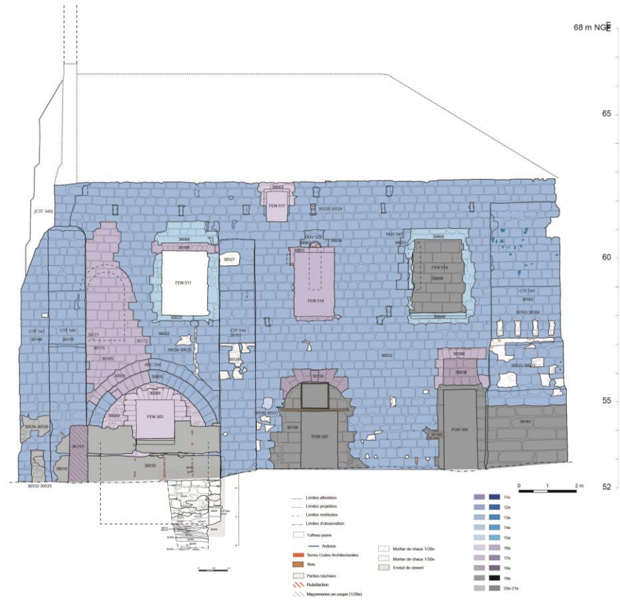
Archaeological phasing of the south façade
